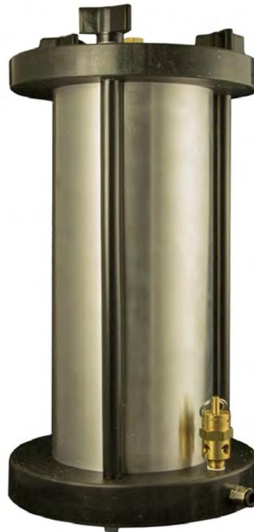
TS1251 pressure pot is designed to accommodate all solvent and epoxy fluids, as well as cyanoacrylates and UV's. Pot accommodates 6mm OD feed tubing with stainless steel compression fittings for a continuous fluid path from the reservoir inside the pot to the metering valve.
